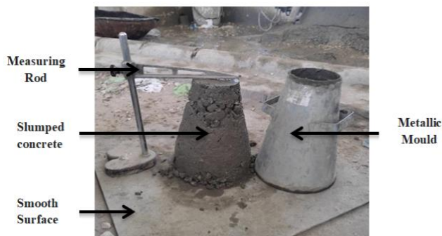
Fig. 2. Setup of Slump Cone Test
