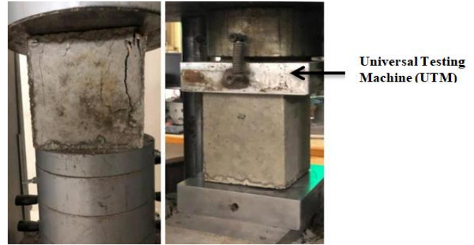
Fig. 4. Concrete cubes under testing
