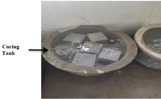
Fig. 3. Curing of specimens for 28 days
