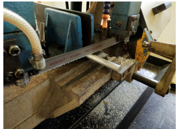
Fig. 3. Cutting Aluminium Rod using Saw Machine
