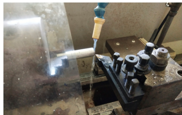
Fig. 4. Shaving Aluminium Rod using Lathe Machine
