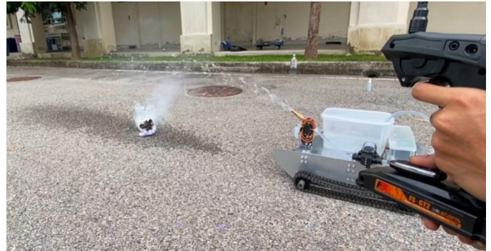
Fig. 7. Controlling water pump with remote
