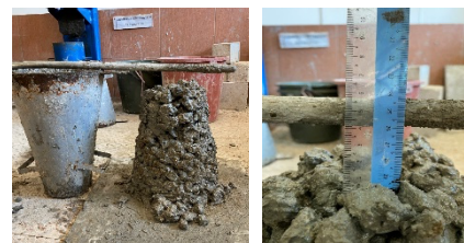
Fig. 2. Measurement of slump height
