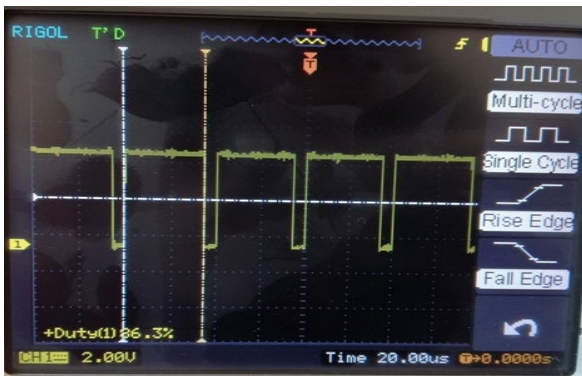
Fig. 11. Pulse width modulation signal generated by ARDUINO UNO
