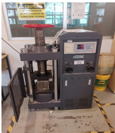
Fig. 6. Compression Testing Machine
