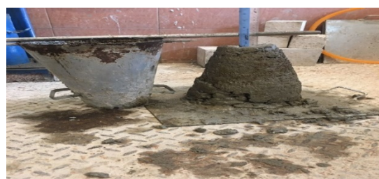
Fig. 4. Obtained Slump Height
