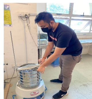
Fig. 2. Conducting Sieve Analysis
