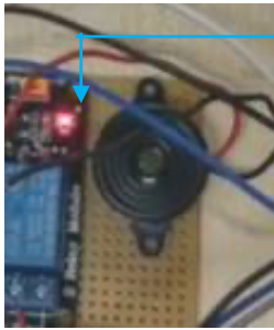
Fig. 9. Relay module switched on upon motion detection.
