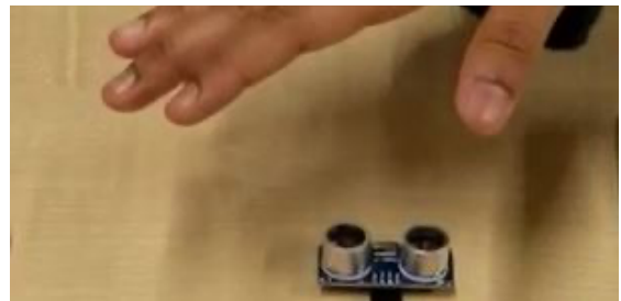
Fig. 8. Motion detection testing by ultrasonic sensor.
