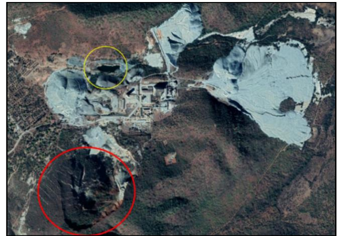
Fig. 2. Observed ground subsidence at Gaths' abandoned mines.
