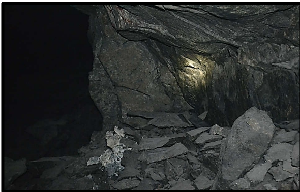
Fig. 16. Preliminary Phases of pillar slabbing
