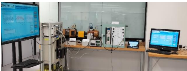
Fig. 7. Photograph of the 3-phase IM full system setup in a laboratory environment with controlled ambient temperature well kept at between 23°C to 25°C
