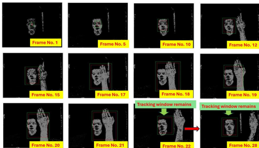
Fig 27. Depicts PD images of enhanced robust and resilient CAMSHIFT algorithm with hand occlusions. Notice the PD images are less noisy as can be seen in the images. The red colour tracking window at frame no. 22 and 28 remains intact with the face and continues to remain stable when the hand slowly moves away from the target face towards the right side.
