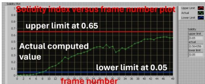
Fig. 17. Depicts the Solidity operator index versus frame number sequence of the processed PD images.
