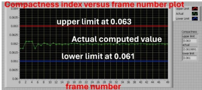
Fig. 16. Depicts the compactness operator index versus frame number sequence of the processed PD images.
