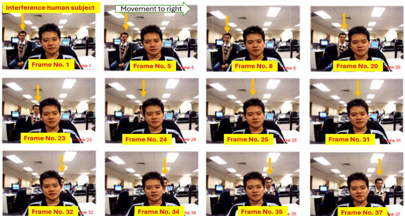
Fig. 29. Depicts occlusion by human subject in the background, moving from left to right direction, tracking is via original CAMSHIFT.
