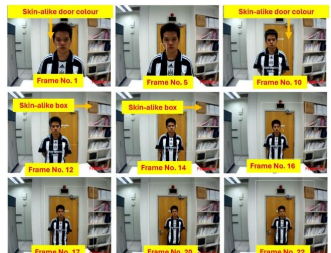
Fig. 41. Depicts RGB images in a video sequence for skin-like background experimentation using Original CAMSHIFT.
