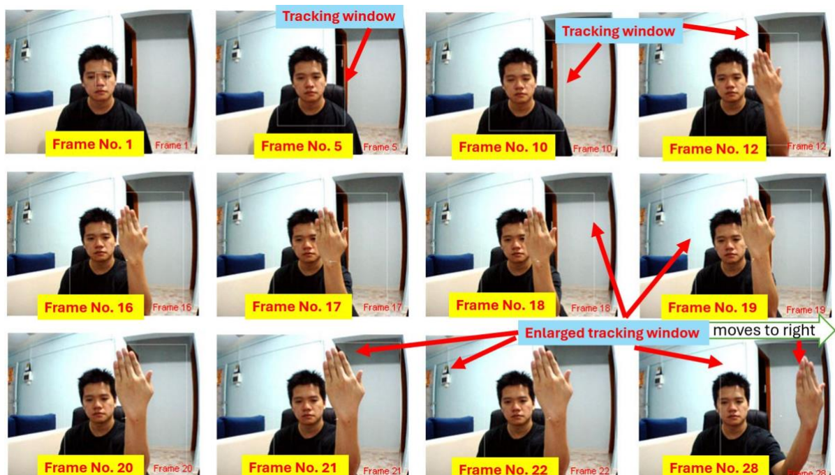
Fig. 25. Depicts RGB images of Bradski's original CAMSHIFT algorithm with hand occlusion. Tracker was unable to differentiate between face and hand occlusion at frame no. 28 based on the enlarge size of the white colour tracking window.
