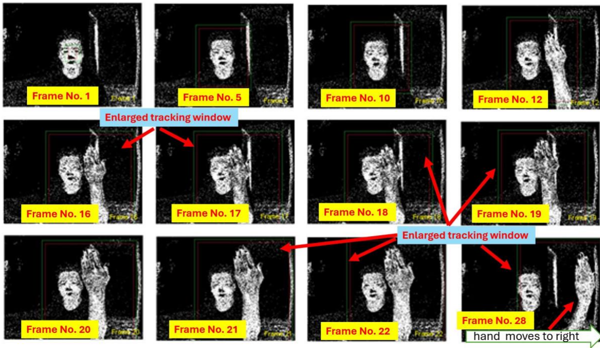
Fig. 26. Depicts PD images of Bradski's original CAMSHIFT algorithm with hand occlusions. Notice the PD images are much noisier as can be seen in the images. Tracker was unable to differentiate between face and hand occlusion at frame no. 28 based on the enlarge size of the white colour tracking window.
