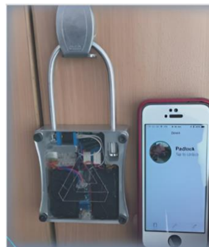
Fig. 6. Entire setup is mounted on the office door (Left), scanning with the phone (Right), Scan the tag here to lock/unlock the door
