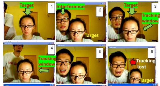
Fig. 24. RGB images in a video sequence using conventional/original CAMSHIFT subjected to a disturbance from an interference face. Tracking was lost on labelled image 6.
