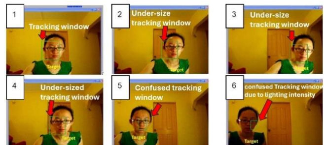
Fig. 31. RGB colour images in a video sequence using original CAMSHIFT subjected to varying lighting illumination.
