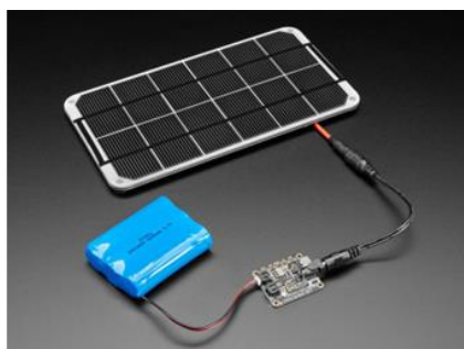
Fig. 1. Example of Solar Buck Converter battery charger.
