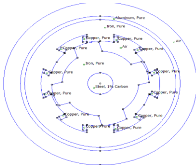
Fig. 2. Section of a type 6/4 switched reluctance machine
