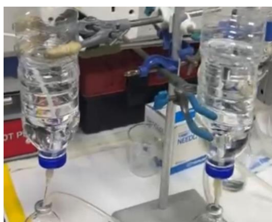
Fig. 1. Experimental setup for CO 2 dissolution by a water displacement method
