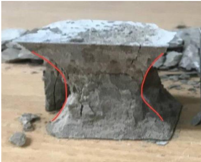
Fig. 6. Failure Mode of Cement Paste Containing Non-Conforming Metakaolin at Various Levels and Curing Periods
