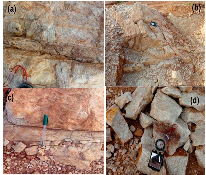
Fig. 10. (a – d) Exposure Quartzite ridge; (a and b) showing different joints/fractures orientation; and (c and d) disintegrated samples
