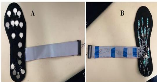
Fig. 3. Smart Insole Layout with Embedded Sensors [10].
