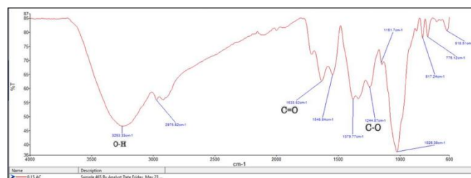
Fig. 3. FTIR Spectrum of AgNPs from A. comosus Peel Extract at 150 mg/mL
