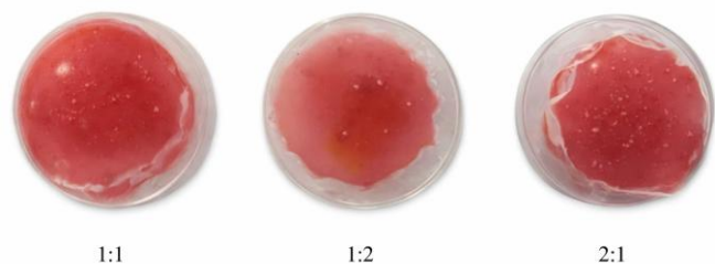
Fig. 3. The Appearance of pH Indicator Films at Different Ratios of Starch to Pectin (1:1, 1:2 and 2:1)
