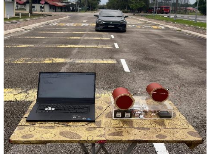
Fig. 10. Outdoor experimental setup of the 2.45 GHz FMCW Doppler radar system used for range and velocity measurements.
