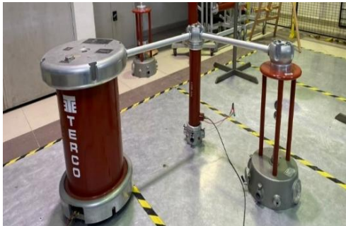
Fig. 3. Dielectric Breakdown Testing Application
