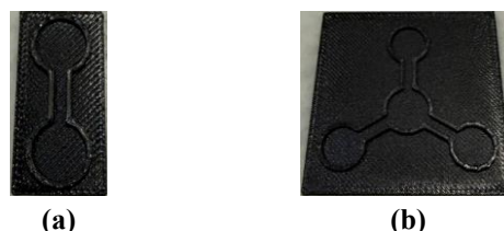
Fig. 5. Fabricated 3D-printed holders. (a) Dual-zone; (b) Y-shaped
