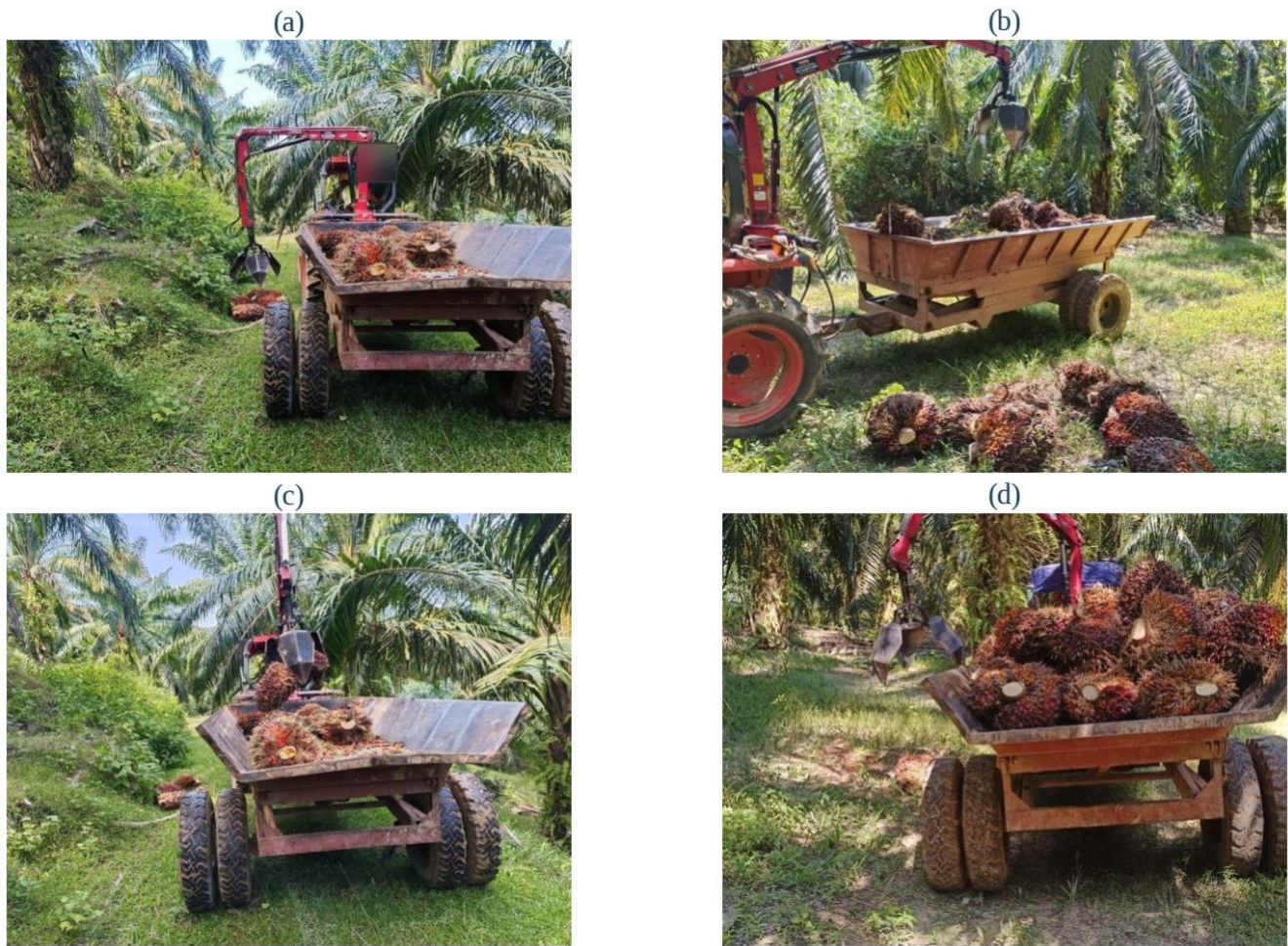
Fig. 2. The MPC unit in routine operation on the study estate: (a) the 45 hp mini tractor with mounted hydraulic grabber and tipping trailer positioned alongside an in-field platform, the vehicle registration masked for anonymity; (b) the grabber lifting bunches from a platform heap into the trailer; (c) a bunch in the grabber jaws being placed into the loaded trailer; (d) a fully loaded trailer at a collection point on a flat block. Photographs taken by the author during the observation period
